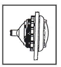
Your QCA Majestic<sup>™</sup> Spa has a standard 12v light. The Spa light may be turned ON or OFF by pressing the Light button located on the spa side control.
