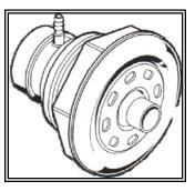
Volcano Jet – the volcano jet is operated by a diverter valve. It is a high velocity jet that increases the water flow up to 20%. To utilize pop the nozzle out. The diverter valve to turn jet on is located on the right side of the steps.
