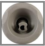
Jumbo Swirl Jet – the water pattern of this Unique jet is adjusted by placing the nozzle into one of the five positive lock positions. The amount of water flow may also be adjusted from full On position to 60% shut-off by rotating jet face clockwise.
