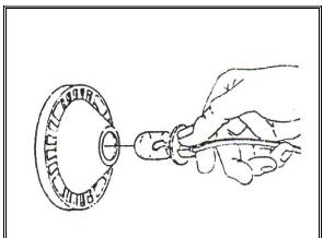
your spa equipment pack. A drain fitting (if equipped) is provided on cabinet panel. Remove plug from drain. Attach garden hose to drain adapter and lay out garden hose to the location where water is to be drained. Screw drain adapter into drain fitting spa will automatically drain by gravity.
